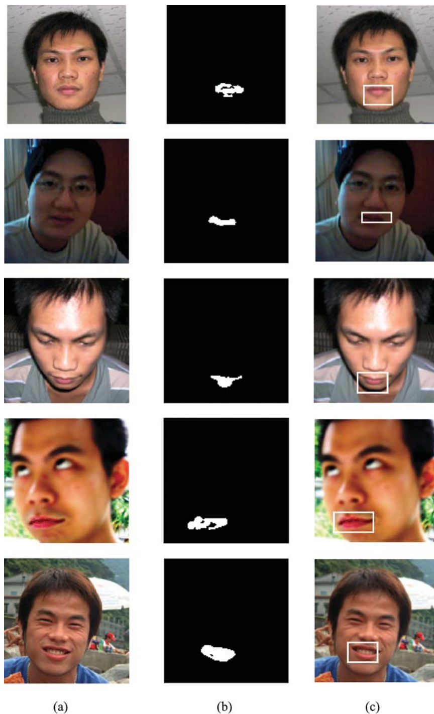
FIG. 11—Some experimental results of face images without masks: (a) the original face images; (b) the mouth blocks; (c) the results. We use a white block to mark the mouth area.
